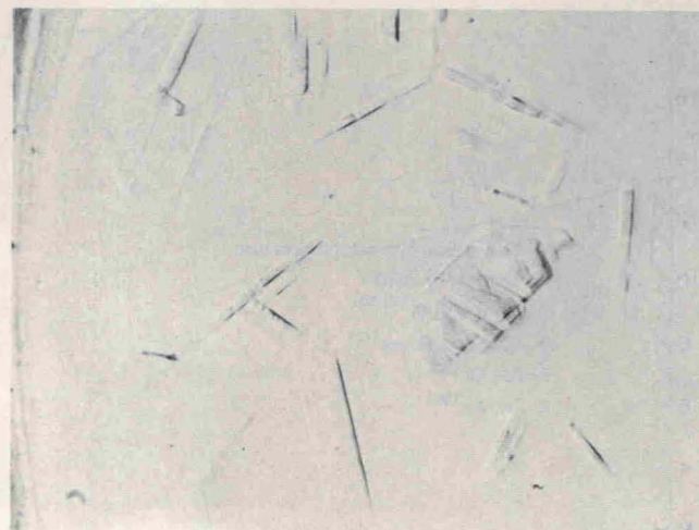
Fig. 7—Fe-11.6 pct Ni-17.4 pct Cr alloy after pressurization. The area is that outlined in Fig. 6(c). Oblique light. Magnification 375 times.
